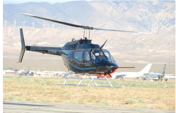
Bell OH-58C (2), Single engine turbine helicopter, Night vision goggle compatible, Instrumented for Performance and Flying Qualities.
