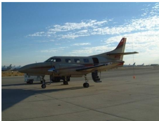
Swearingen SA-226 Merlin II , Instrumented for Performance and Flying Qualities, Twin turboprop commuter aircraft.
