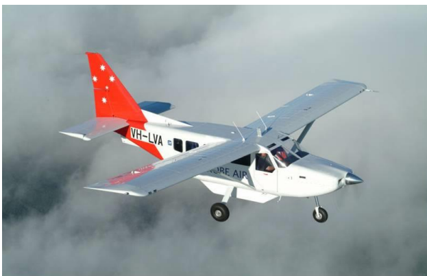
Gippsland GA-8 Airvan , Single engine recip, Night vision goggle compatible, FLIR and Weather RADAR equipped.
