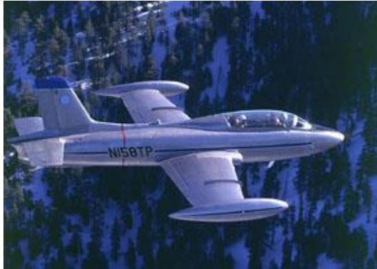
Aermacchi MB-326 Impala (5). Single engine jet trainer, Instrumented for Performance and Flying Qualities (1 AC), Spin test training, Upset training, Loads and flutter TM system (1 AC).
