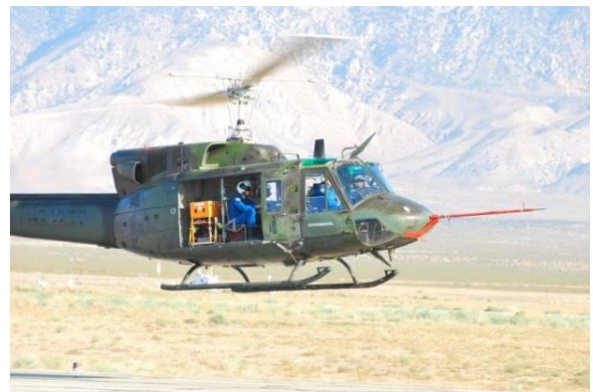
Bell UH-1N Huey , Twin engine turbine helicopter, Night vision goggle compatible, Instrumented for Performance and Flying Qualities, LORAS / FLIR, SAS & Auto Pilot.
