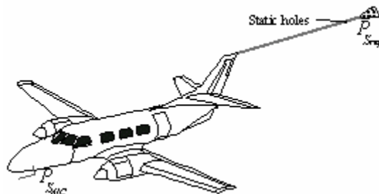
Figure Error! No text of specified style in document. -25 Trailing Static Cone
