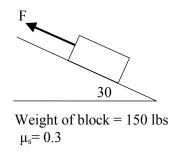
Find: a) Minimum force required to hold the block at rest.
