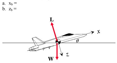
Given the following, resolve **W** onto the body axis and determine the following equations
