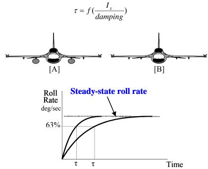
Match the roll mode time constant with the appropriate configuration.
