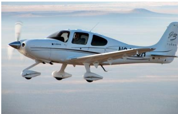
Cirrus SR22 (3) , Single engine, piston propeller, Sidestick controls for pitch and roll, Emergency Airframe Parachute System, Dual Garmin 430 navigation systems (1 AC), Large multifunction display (Avidyne FlightMax) (1 AC) Garmin 1000 Avionics (2 AC).
