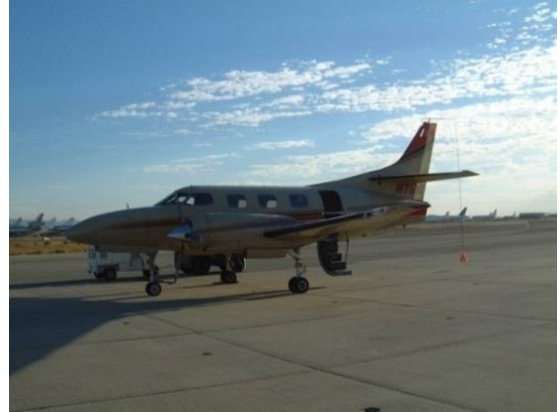
Swearingen SA-226 Merlin II , Instrumented for Performance and Flying Qualities, Twin turboprop commuter aircraft.
