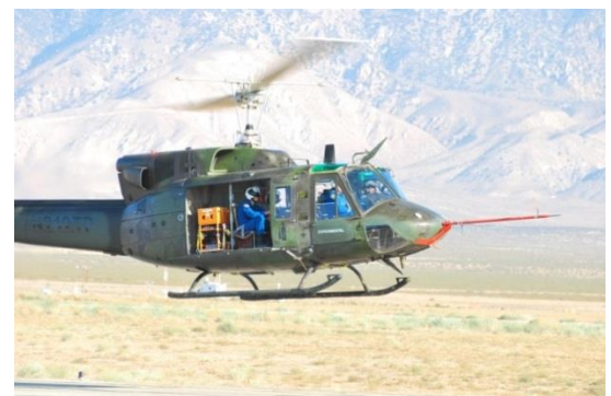
Bell UH-1N Huey , Twin engine turbine helicopter, Night vision goggle compatible, Instrumented for Performance and Flying Qualities, LORAS / FLIR, SAS & Auto Pilot.
