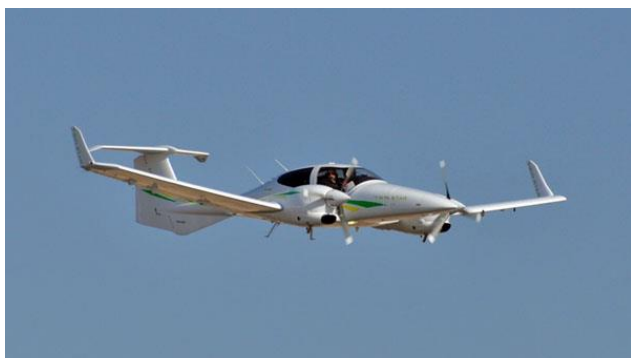
Diamond DA-42 (1) , Twin engine FADEC diesel, OEI Flight test demonstrator.
