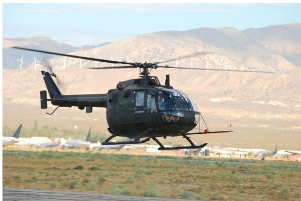
MBB BO-105M (2) , Light weight, twin-engine, multipurpose helicopter, Instrumented for Performance and Flying Qualities.
