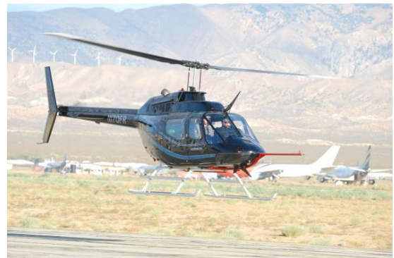
Bell OH-58C (2), Single engine turbine helicopter, Night vision goggle compatible, Instrumented for Performance and Flying Qualities.
