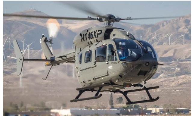
Airbus Helicopters EC-145 , Twin engine light utility helicopter used for RW P&FQ and Systems testing.
